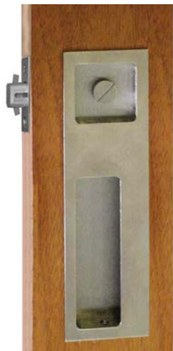
SET: 13.PA906I Passage set with tubular lock with flush escutcheon with pull cup; minimum door thickness: 1 3/4" SET: 13.PR906I Privacy set with tubular lock with flush escutcheon with pull cup; minimum door thickness: 1 3/4"
