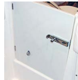
#44.0604 Transom bolt / barrel bolt; Body: 100 X 32 X 12 mm; 4" x 1 1/4" x 1/2"; Throw: 7/8" 316 stainless steel Strike flush #44.0605; Strike angle #44.0606 EXCELLENT FOR BULWARK DOORS
