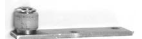
#54.281 bottom guide wheel for sliding door. Plate stainless steel 23 x 100 mm; 4 mm thick. Diameter nylon wheel: 19 mm or 3/4 inch.
